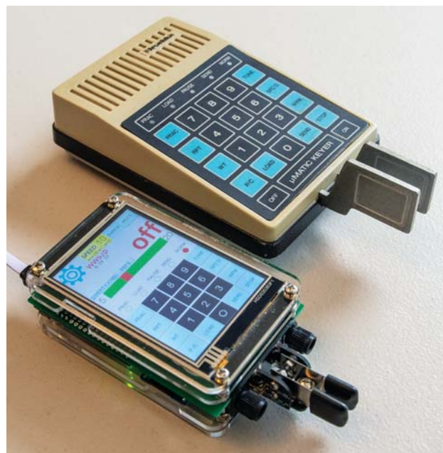
Figure 1 — The WW9JD Arduino-based \mu Matic2 Memory Keyer next to the original Heathkit SA-5010 \mu Matic Memory Keyer.
